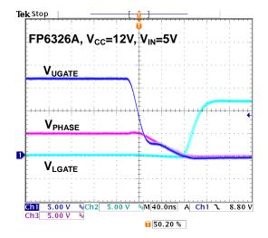
Figure 14. Switching waveform (UGATE Falling) I<sub>OUT</sub>=0A
