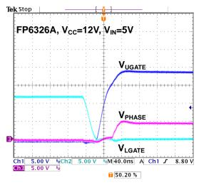
Figure 13. Switching waveform (UGATE rising) I<sub>OUT</sub>=15A
