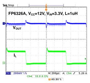
Figure 23. Transient test:1kHz, Slew rate:2.5A/us
