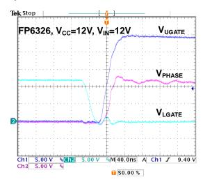
Figure 16. Switching waveform (UGATE rising) I<sub>OUT</sub>=0A
