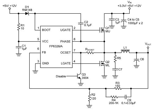
Figure 2. Typical Application Circuit of FP6326/A
