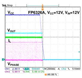
Figure 11. Power OFF at 15A Loading
