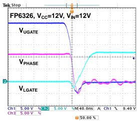
Figure 18. Switching waveform (UGATE Falling) I<sub>OUT</sub>=0A
