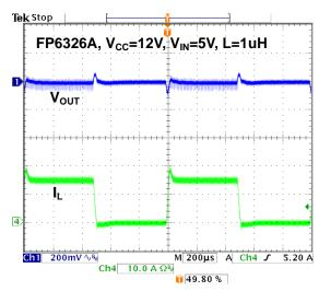
Figure 22. Transient test:1kHz, Slew rate:2.5A/us
