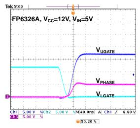
Figure 12. Switching waveform (UGATE rising) I<sub>OUT</sub>=0A
